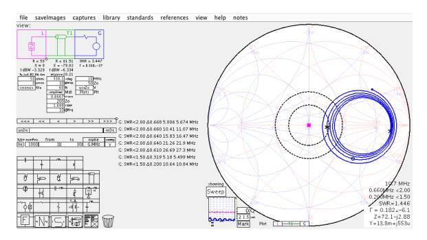
In the above, the extra information offered up is the frequency ranges which fall below the SWR circles specified on the Smith chart. This is the only information presently displayed automatically.
