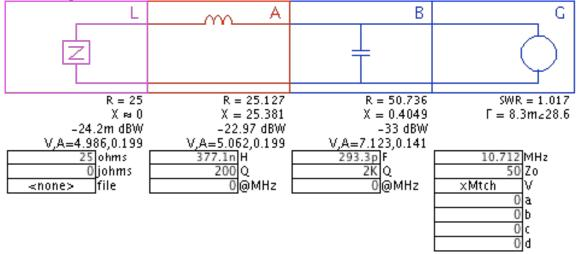
This is a simple LC impedance match from 25 ohms to 50 ohms at 10 MHz. The generator V equation is using the 'xMtch' builtin which ensures that, regardless of the circuit impedance, 1 watt will be
