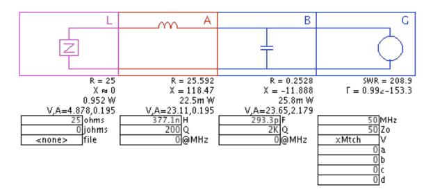
Here, the 'xMtch' must adjust the voltage upward significantly in order to deliver 1 watt to the circuit: now 23.6 volts instead of only 7.07. The load gets .952 watts and the LC circuit dissipates 50 milliwatts. The components are not very lossy so the majority of power still gets to the load but the generator must (and does) compensate for the large impedance mismatch.
