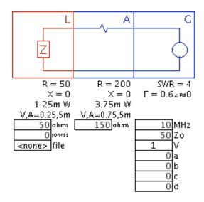
Notice that the voltage of L is .25 volts and the voltage across A is .75 as expected. Note that the current through both resisters is the same. This is, by far, the easiest use of the generator equation and is generally adequate for most situations. There are, however, times when the generator voltage must vary.
