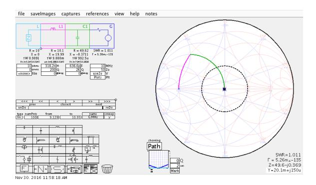
Notice that SimSmith traces the path of the impedance as it progresses from the load (at 10 ohms), through the series inductor (in magenta) and past the capacitor (green). The 'showing' field indicates the display
