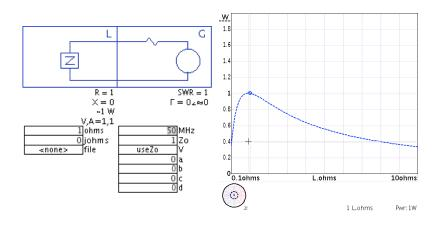
Now, understanding the 'maximum power transfer theorem' we can see how it might be used. Suppose we have a generator with a 50 ohm internal impedance and a load of 25 ohms. What is the total power delivered to the load in this mismatched case?
