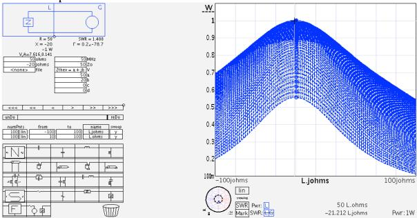
Note that the maximum occurs when the 'Load' is the "complex conjugate" of the generator internal impedance.
