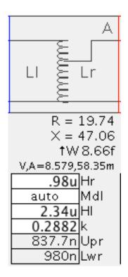
When using the 'auto 'model, the transformer consists of a single coil with two taps. As with the isolation transformer, the auto transformer requires the specification of the inductance of the two taps and the coupling coefficient 'k'. SimSmith requires that the k be  $\geq 0$ . It is allowed to be larger than 1 but that makes the transformer 'non-physical'.
