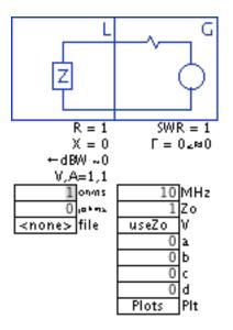
If the 'maximum power transfer theorem' is true, we should get maximum power when the load 'L' is 1 ohm as well. SimSmith can be used to verify this by scanning over a range of values for L. Here is a plot of the power being dissipated by L:
