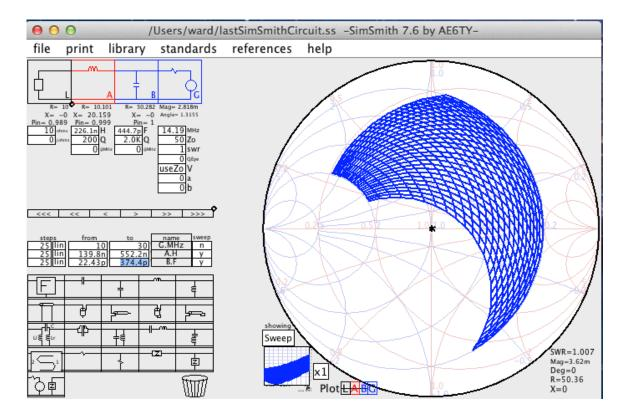
During a sweep, the steps can be equally spaced (lin) or logarithmically spaced (log). You can select which is being used by clicking on the button in the 'steps' column. Of course, you can change the lower and upper bounds of the scan and the number of steps to take. You can even reverse the direction of the scan if you wish.
