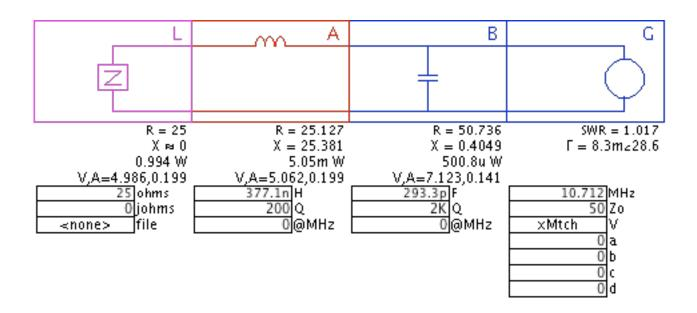
Thus, 'xMtch' is delivering 1 watt and .994 is going to the load and .00505 + .0005 watts is being dissipated by the LC match.
