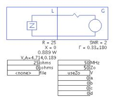
As it turns out, the 25 ohm load will receive .889 watts in this case; only about 10% down from the theoretical maximum of 1 watt.
